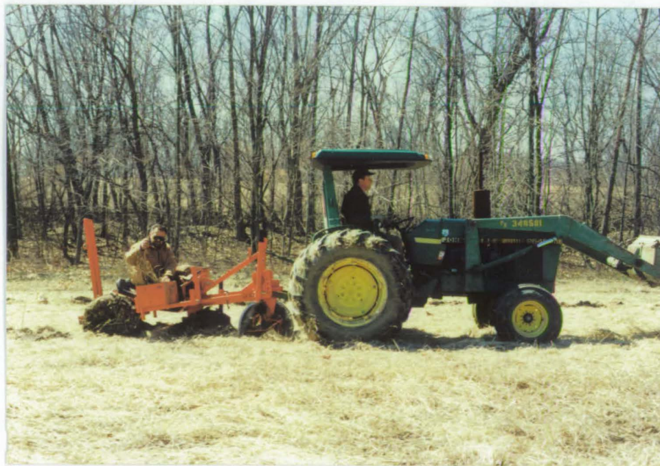
Tractor Operator Lagemann and Maintenance Mechanic Milazzo used the new seedling planter to plant a variety of bottomland species in fields on the Delair Division.
