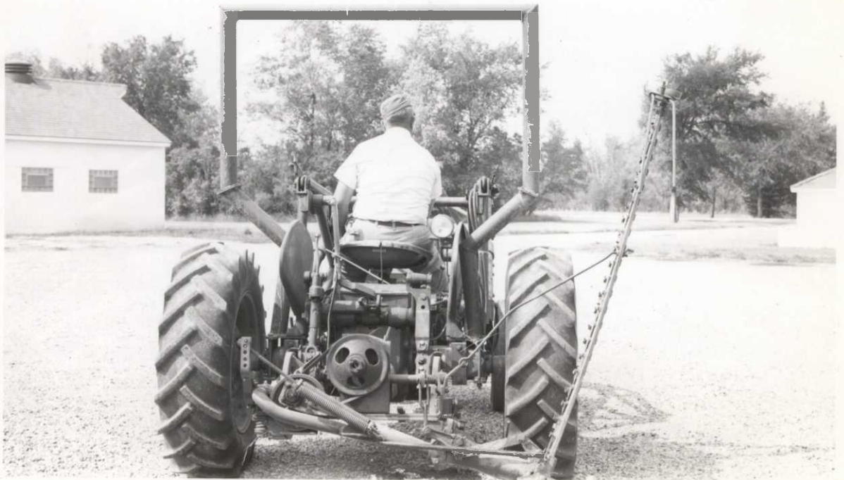
Safety Roll Bar attachment for wheeled tractors. This suggestion won $50 for Mgr. Ed Smith. Photo by EJS.
