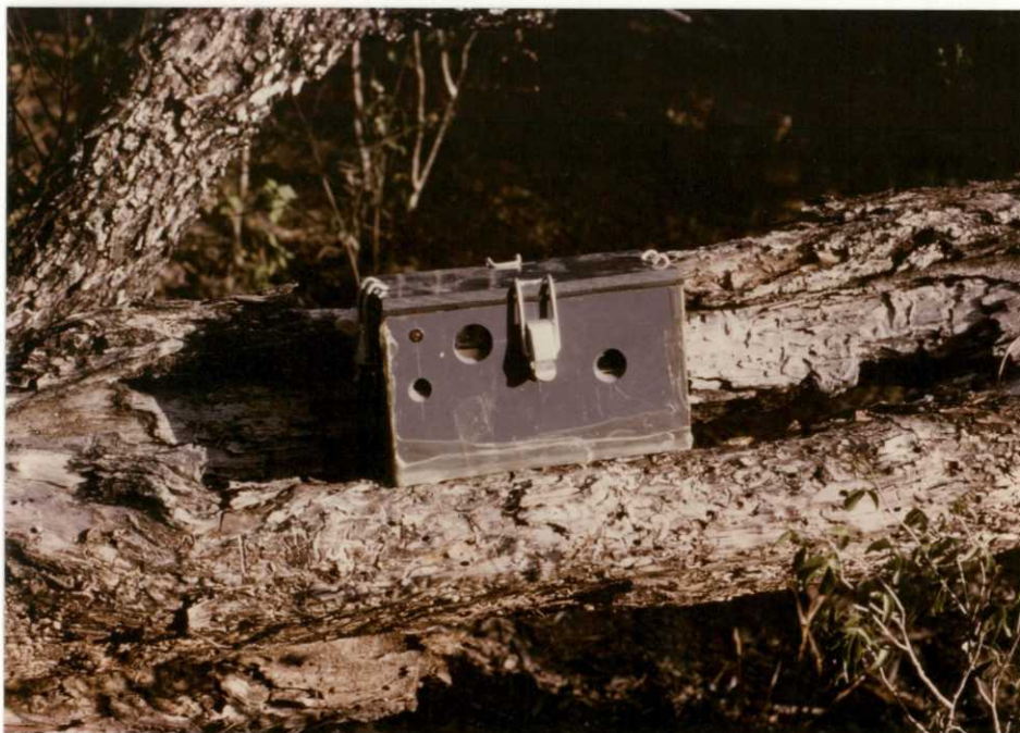
An infrared trip beam camera case is posed for your viewing. The infrared source box appears in many of the wildlife photographs. An animal moving between the two boxes breaks the beam and takes its own photograph. (14MR86, JI)
