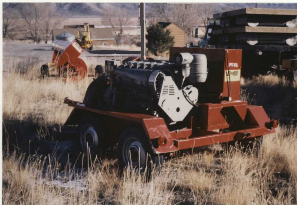
Figure 32. the air cooled Deutz diesel engine purchased with Special Congressional Appropriated Funds. SMB 12/87
