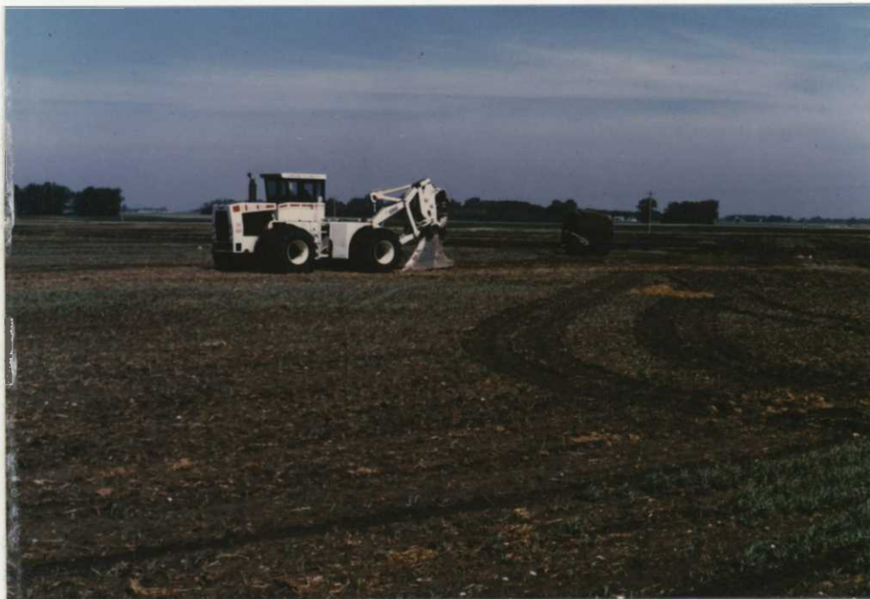
Big Bud, as this machine is affectionately known by those it serves, is a graphic example of current drainage capabilities. Note the large roll of tile in the background.
