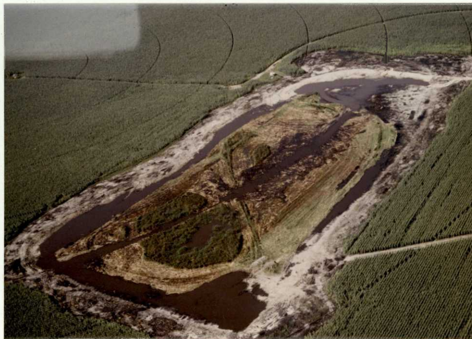
Hauge Easement (43X) Pope County, a filling violation where earthen fill was placed within the high water mark in order to farm closer to the basin. 81-16 DEM
