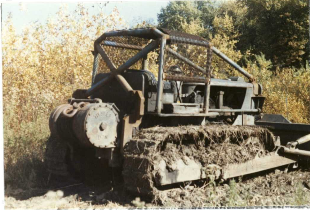
ROPS reinforced by Pennington Welding, Waukomis, Oklahoma. Total cost for the job was $3,245 and no certification. Welder misunderstood a portion of the static load testing required by OSHA. (R-970, P-20, TSS) (10-29-84)
