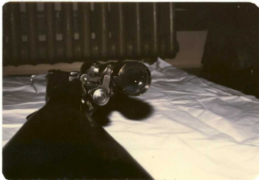
Closeup view of the safety on the above Springfield rifle Model 1903-A3 showing the obstruction caused by the scope lens. Safety tang must be turned clockwise to the 3 o'clock position to be fully safe. Low mounting of the scope with no modification of the safety tang allowed tang to be raised only to near 11 o'clock position. Note the wire through the forearm used to hold the sling's front end in place. November '76. C.S. Peck
