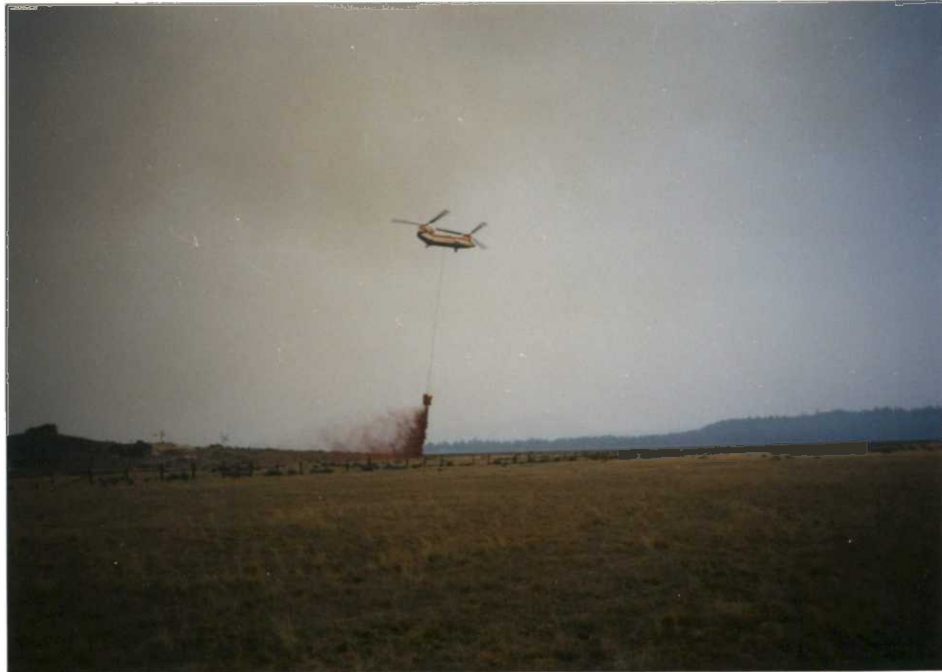
Heavy helicopter (chinook) laying down retardant around structure in advance of fire spread on Lone Pine Fire.
