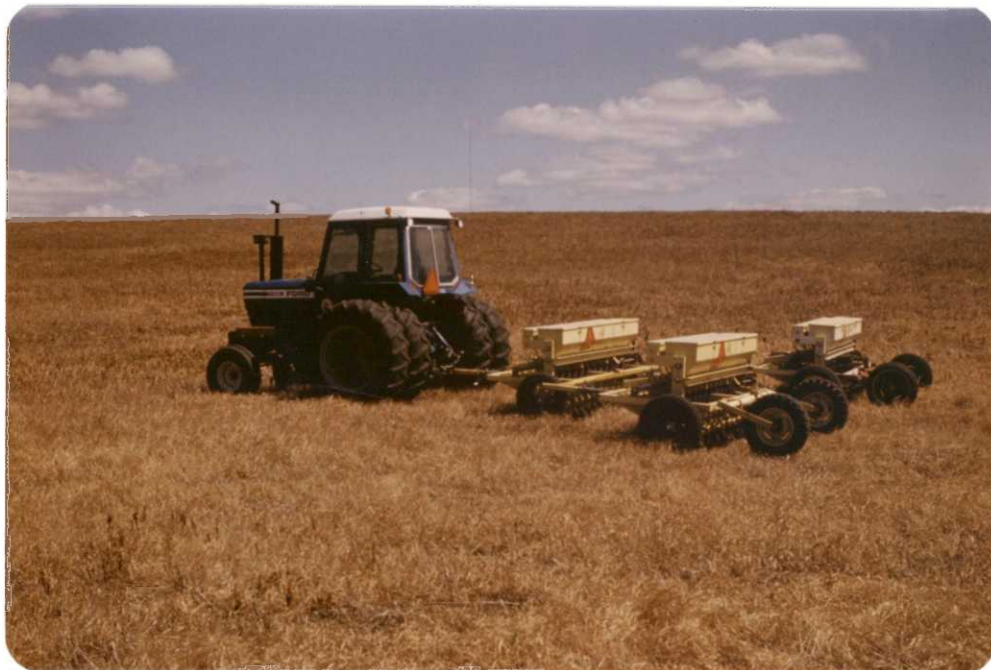
This modified 3-drill hook-up allows us to seed many acres of native grass in one day.
