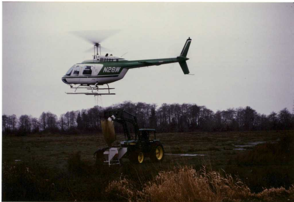
#5-Loading of the aerial fertilizer bucket with fertilizer for application on Miller Sands and Rice Islands. 89-RTV
