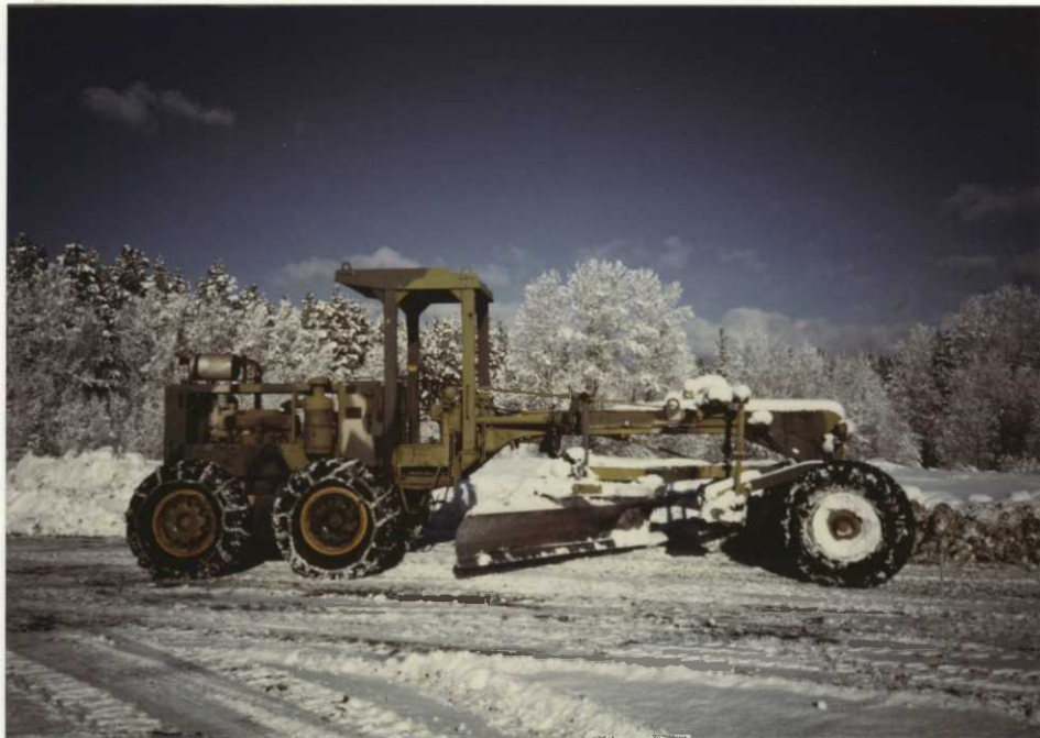
#10-Caterpillar (1964) Model 12 grader was received excess from Fort Lewis to replace 1953 Austin-Weston. Note air conditioned cab insures 'quick' work of winter snow-plowing jobs. 86-HEC
